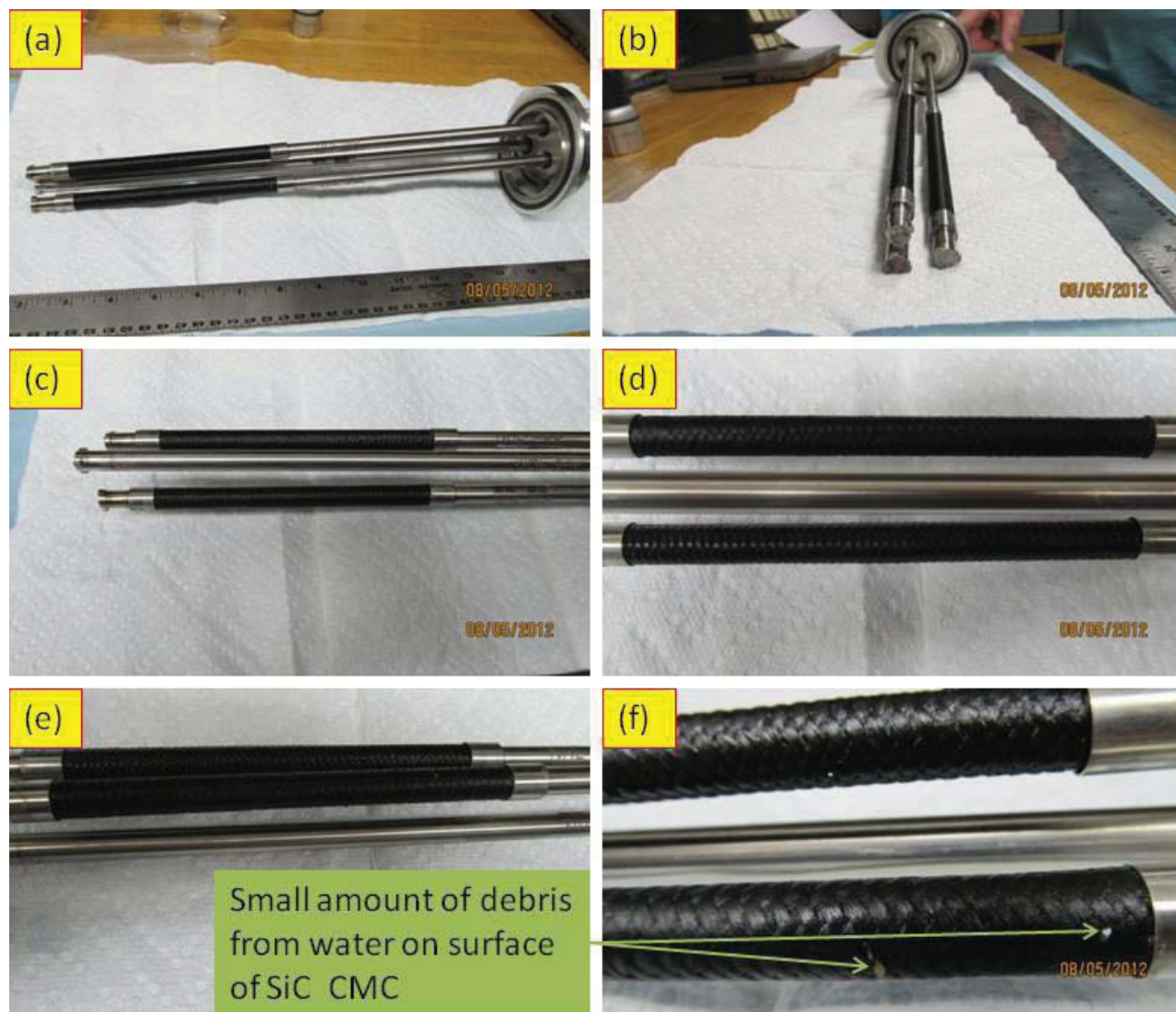
Figure 16. Photographs of Zr-4, SiC CMC rodlet samples following a three-day test run at 125°F. (a) Longitudinal view. (b) End-on view. (c-f) Various longitudinal views. (f) A small amount of debris from water collected on SiC CMC. No corrosion of Zr-4 was observed.
