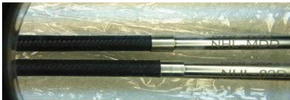
Figure 19. Magnified visual examination shows no evidence of corrosion products on the 2 hybrid CMC and Zr-4 test samples. Note that minor particulate debris on the CMC samples was removed at 3-days prior to re-insertion for the remainder of the 10-day run.
