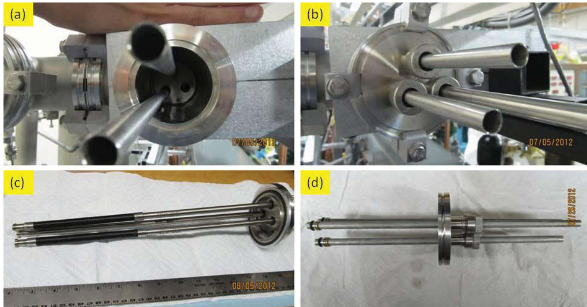
Figure 5. (a) Two rodlet samples are placed inside flow channels of basket. (b) Rodlets adaptor flange installed in system. (c) Two SiC CMC samples and one Zr-4 sample after removal from system. (d) Diagnostic tool used to measure flow through each of the basket channels.
