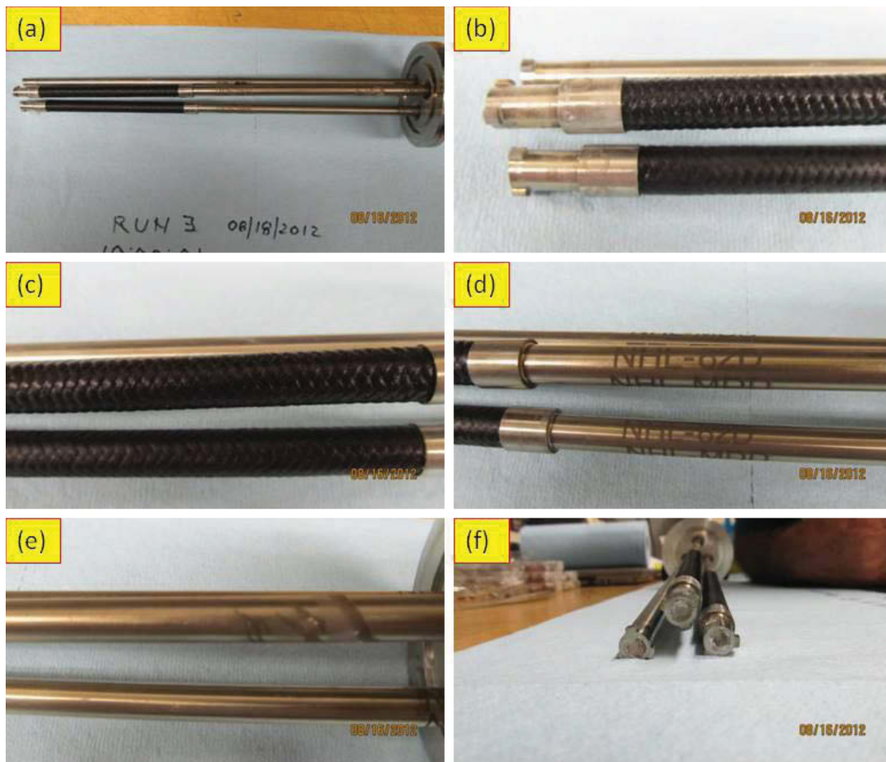
Figure 18. Photographs of Zr- 4 and SiC/CMC rodlet samples following the ten-day test at 125°F. (a) Sample holder removed from system. (b) Upstream end of samples. (c) Center of samples. (d,e) Downstream end of rodlets. (f) Edge view of rodlets.
