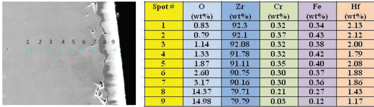
Figure 5. EDS element probe data taken on a Zr-702 sample following one hour exposure to air/supersaturated steam at \sim 1000^{\circ}\text{C} . (a) SEM photomicrograph showing sampling locations. (b) Wt.% data for O, Zr, Cr, Fe and Hf at various sampling locations.
