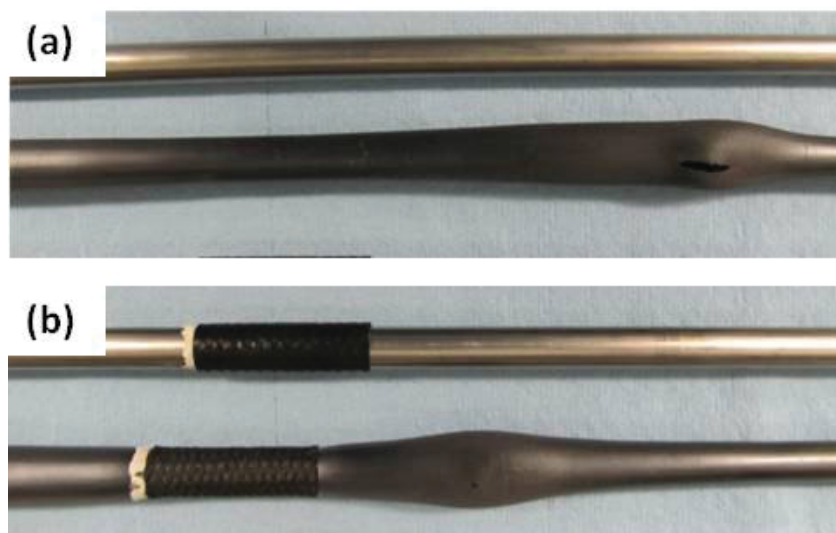
Figure 8. Photographs of starting samples (above) and ruptured samples (below) of (a) Zr-702 tube, and, (b) Zr-702 tube fitted with a SiC CMC sleeve.
