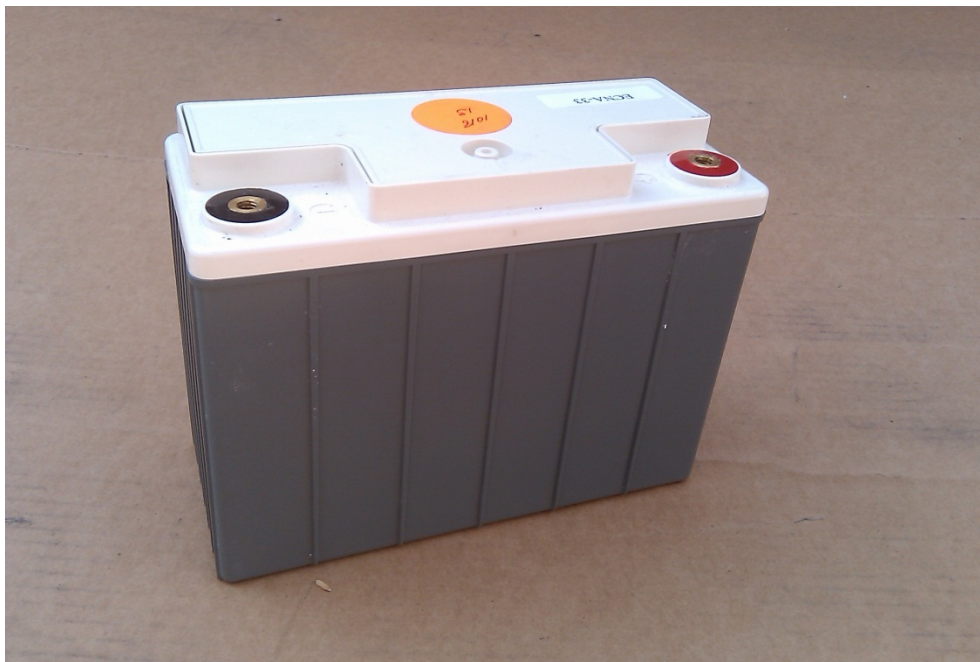
Figure 53. Picture of a 12-V, 10-Ah, Advanced Lead-Acid Battery Consortium high-carbon battery.
