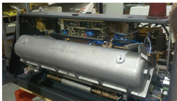
Figure 1. Optical cavity houses the slab and is equipped with sight glasses.
