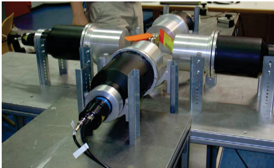
Figure 14 Side-view photograph of the three plutonium samples, within a lead sleeve, centered between the four liquid-scintillator detectors.
