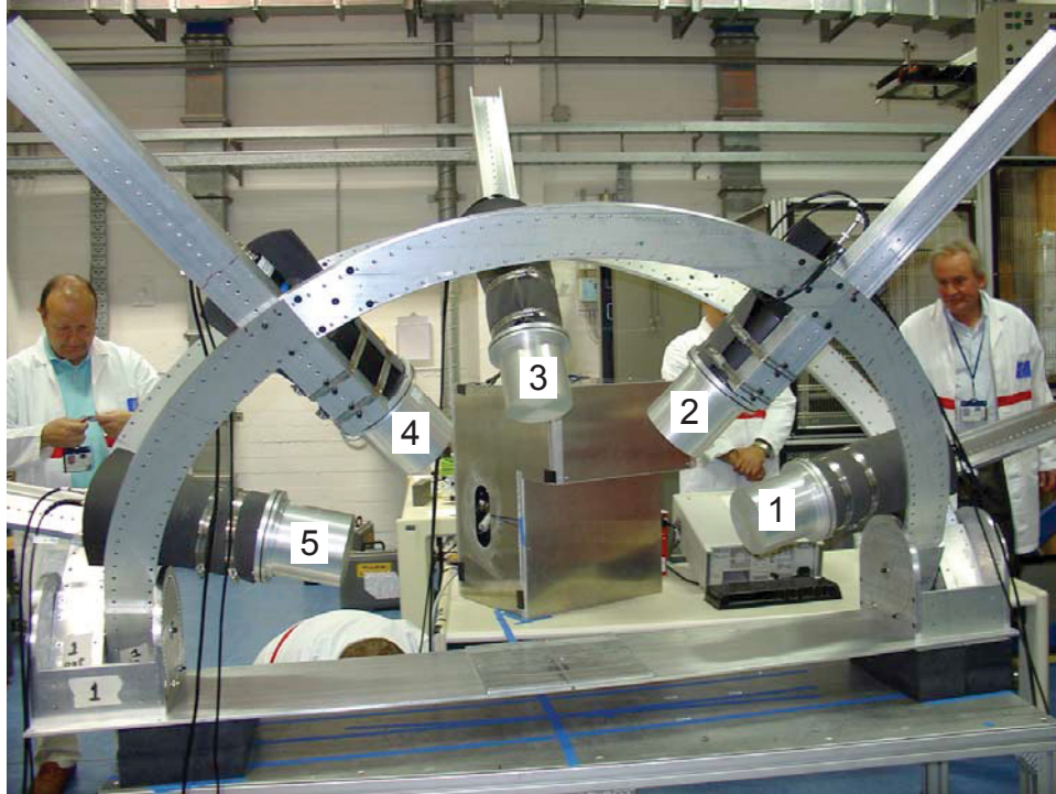
Figure 9 Photograph of the liquid-scintillator array positioned in front of the AP-ENG for a background measurement.
