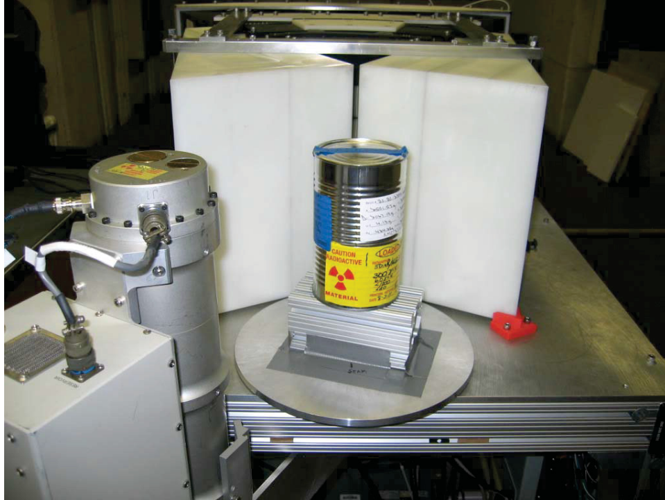
Figure 40 Photograph of an inspection object in front of the radial collimator – end view.
