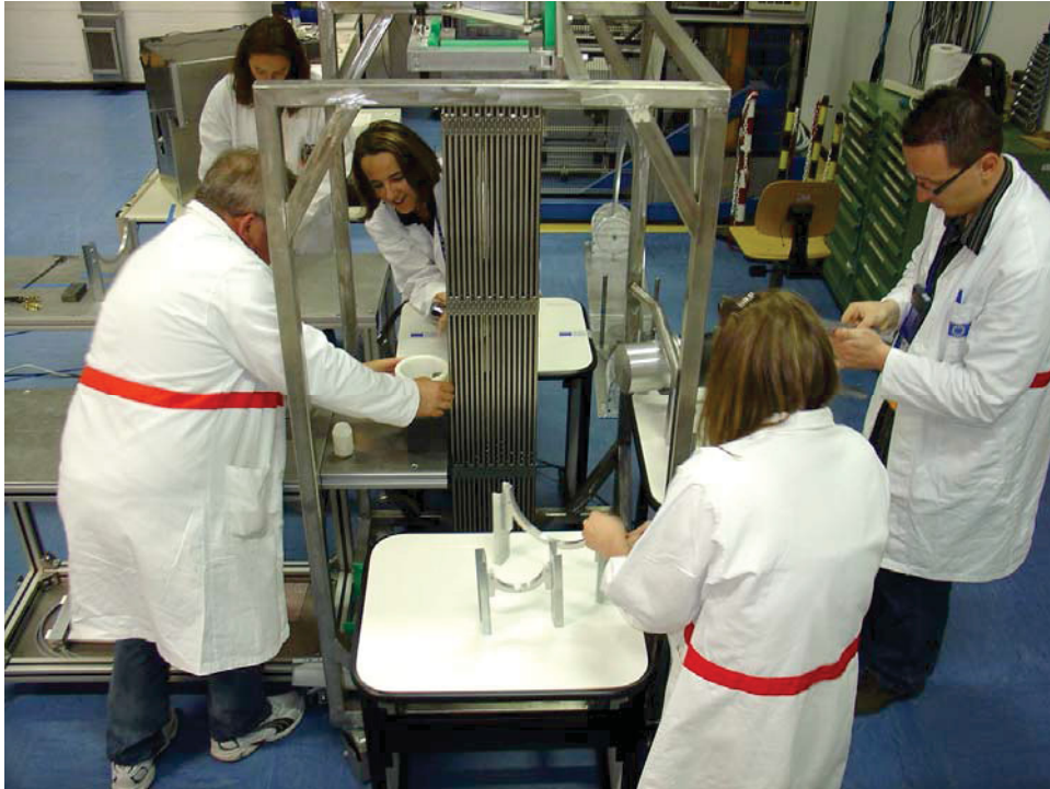
Figure 15 Photograph showing the detectors being arranged on three sides of the PWR fuel assembly, with cylindrical polyethylene and lead sleeves being positioned to receive the AmLi source.
