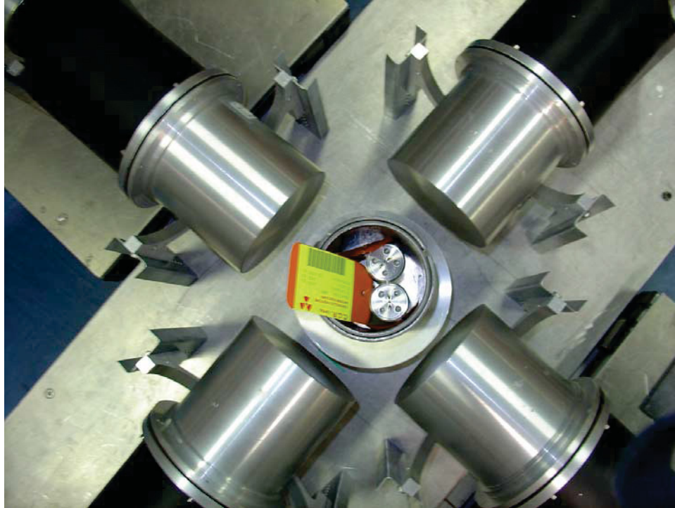
Figure 13 Top-view photograph of the three plutonium samples, within a lead sleeve, centered between the four liquid-scintillator detectors,
