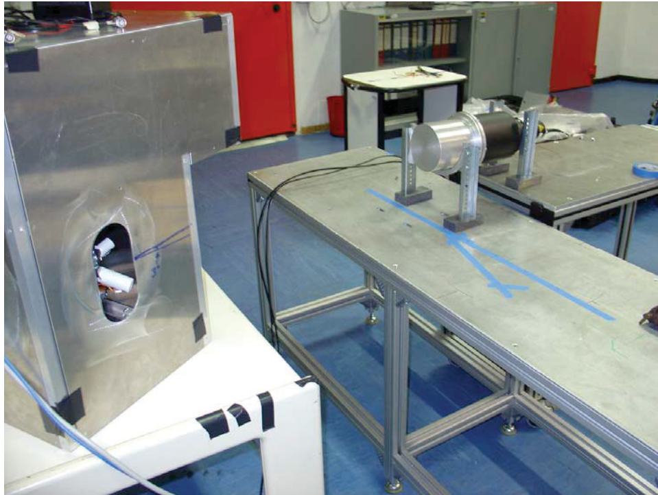
Figure 7 Photograph of one liquid-scintillator detector in position for scanning the tagged-beam region characterizing the AP-ENG.
