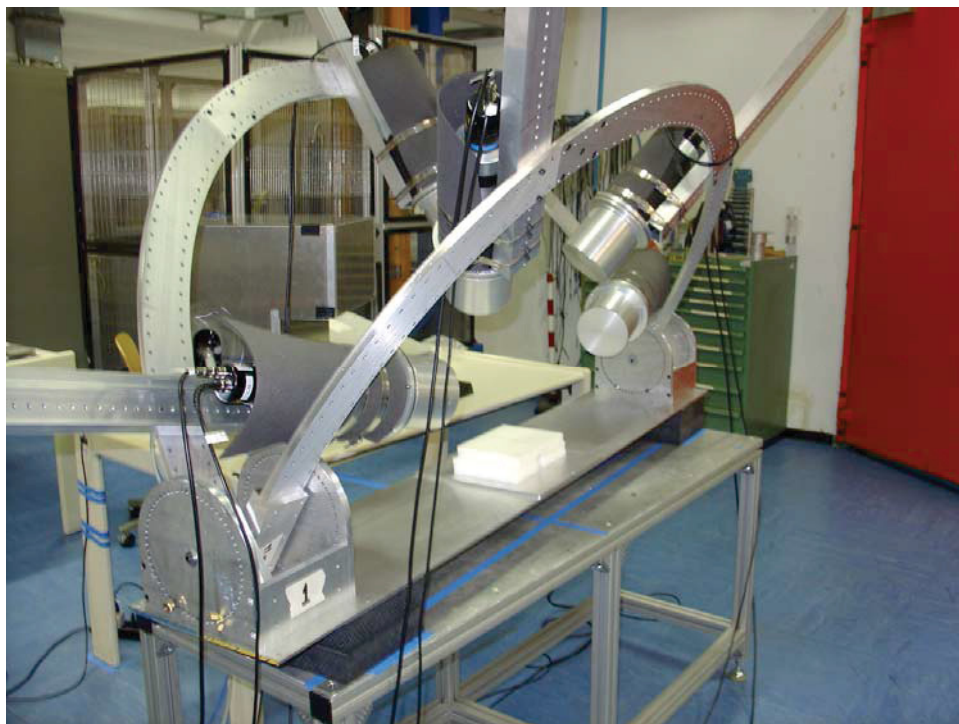
Figure 10 Photograph of the AmLi source positioned within the polyethylene assembly in the detector arch, for collecting the background spectrum.
