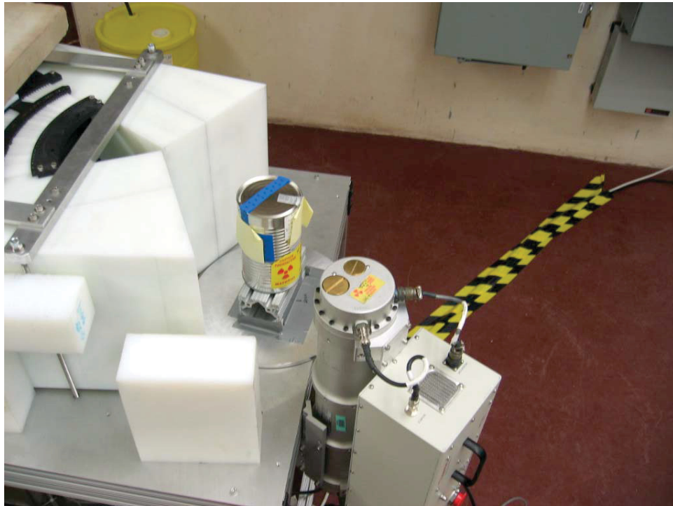
Figure 43 Photograph of an inspection object in front of the radial collimator – top/side view.
