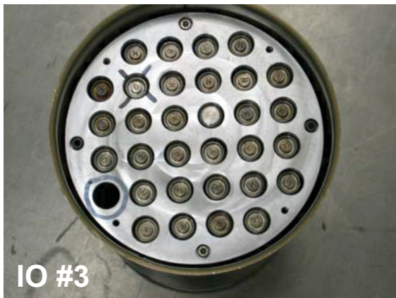
Figure 35 The four inspection objects loaded with pins, prior to final assembly and sealing.
