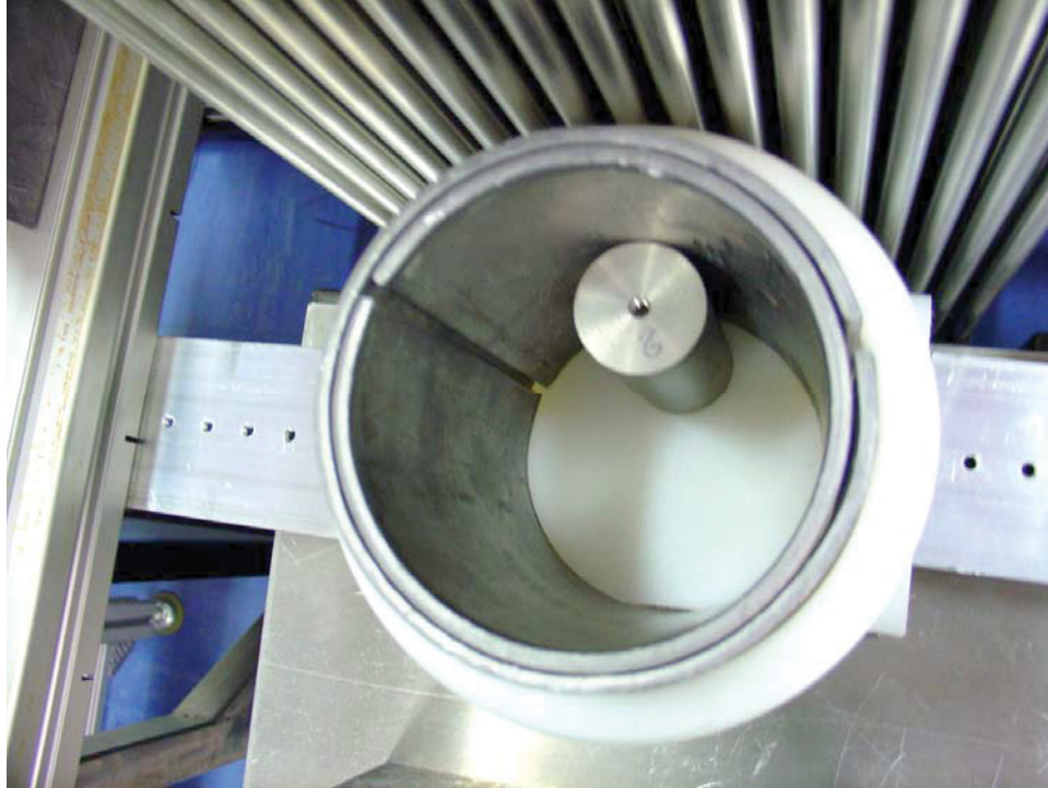
Figure 16 Close-up photo of the AmLi source in the cylindrical sleeves of polyethylene and lead.
