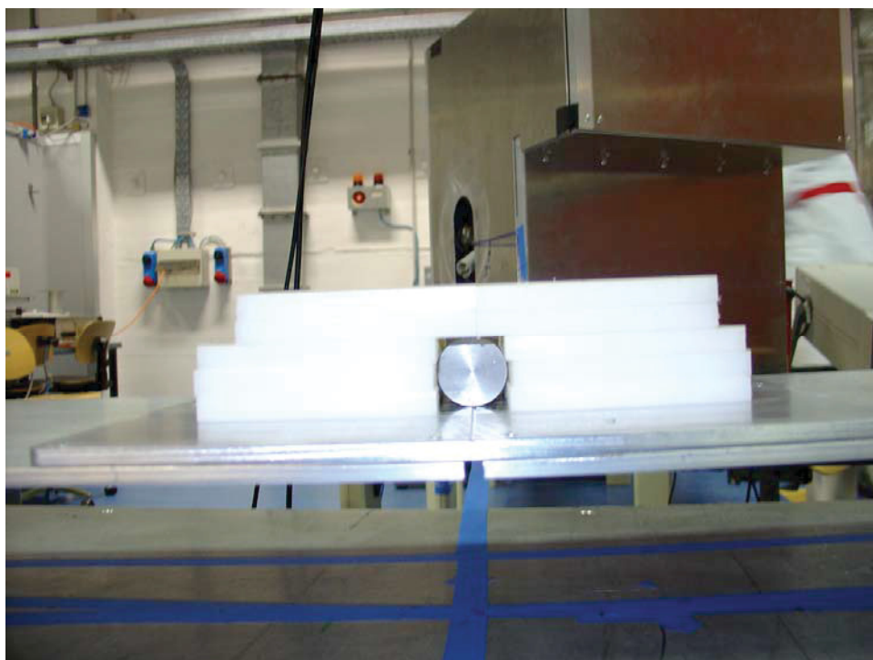
Figure 11 Close-up photograph of the AmLi source in the configuration used for irradiating the uranium oxide fuel.
