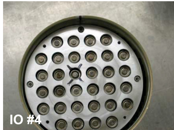
Figure 35 The four inspection objects loaded with pins, prior to final assembly and sealing.
