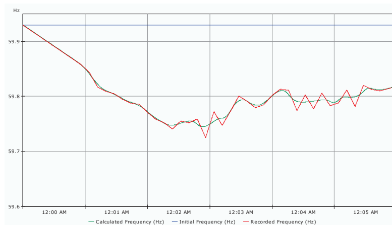
Figure 11. Frequency as a function of time for the simplified MEGS model compared to actual data.
