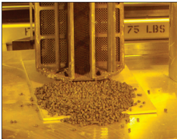
Fig. 2: Undissolved anode materials from the Mk-IV ER
