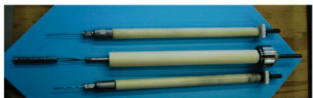
Fig. 3. Stainless steel and platinum wire working electrodes (top and bottom); molybdenum wire counter electrode (center).
