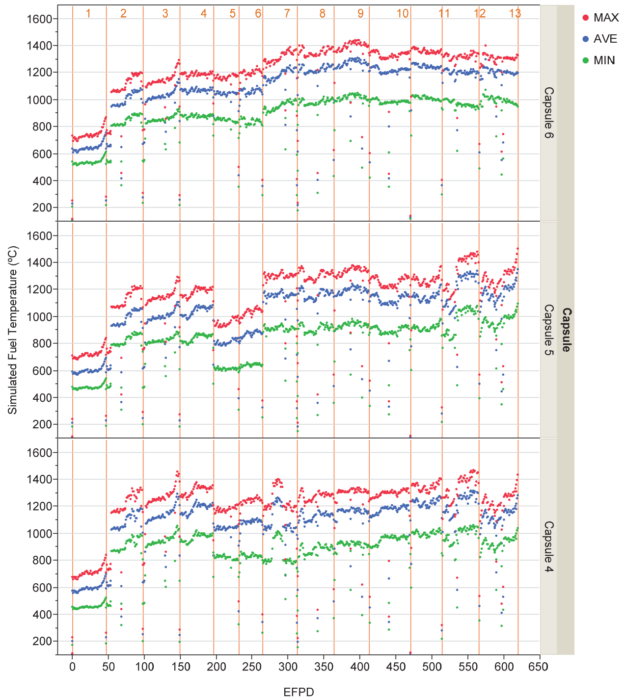
Figure 3-5. Calculated daily minimum, maximum, and volume average temperatures for Capsules 4–6.
