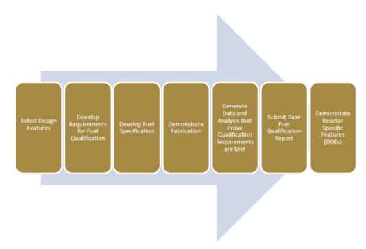
Figure 1 Schematic flowchart showing basic steps for fuel qualification.<sup>2</sup>
