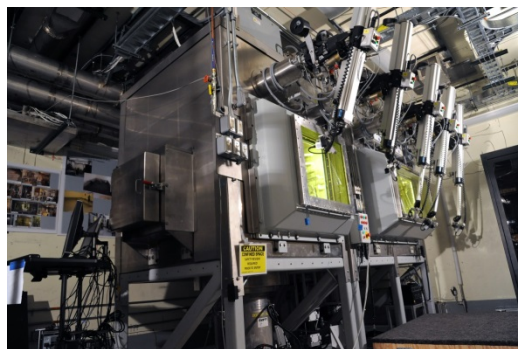
Newly constructed irradiation assisted stress corrosion cracking test rigs.
