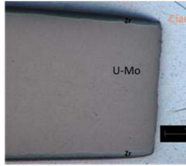
Figure 85. Plate L5P3B1, mount 51V. Average fission density: 2.49\text{E}+21 \text{ f/cm}^3 . Low-fission-density micrograph of cladding/U-Mo interaction layer (thick fuel meat plate).
