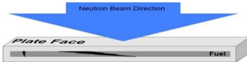
Figure 10. Resolvable cracks in fuel using a configuration perpendicular to plate face.
