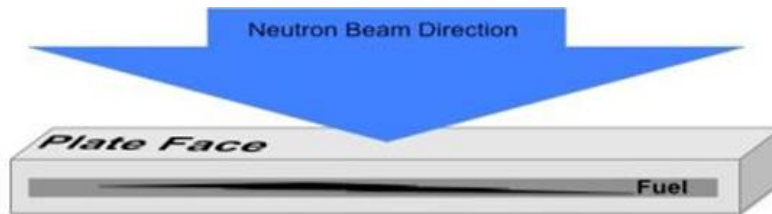
Figure 11. Non-resolvable crack in fuel using a configuration perpendicular to plate face.
