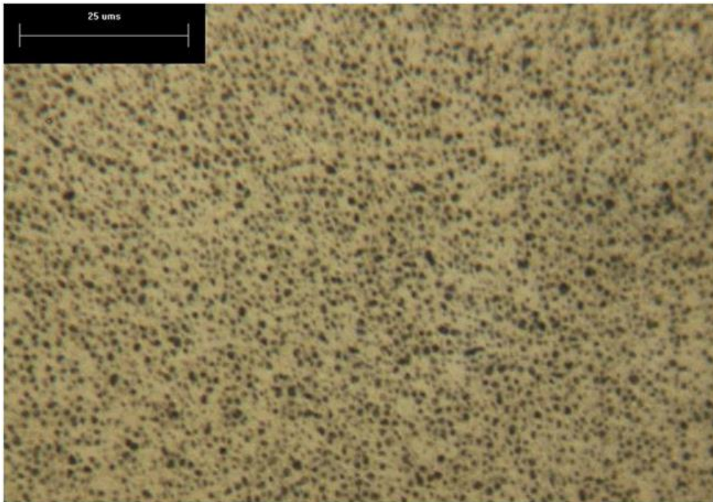
Figure 60. L1P784, mount 44V. Average fission density: 6.3 \times 10^{21} \text{ f/cm}^3 . Optically resolvable grains have been almost completely transformed. Fission-gas bubbles are coarsening, and incipient interconnection of bubbles is evident.
