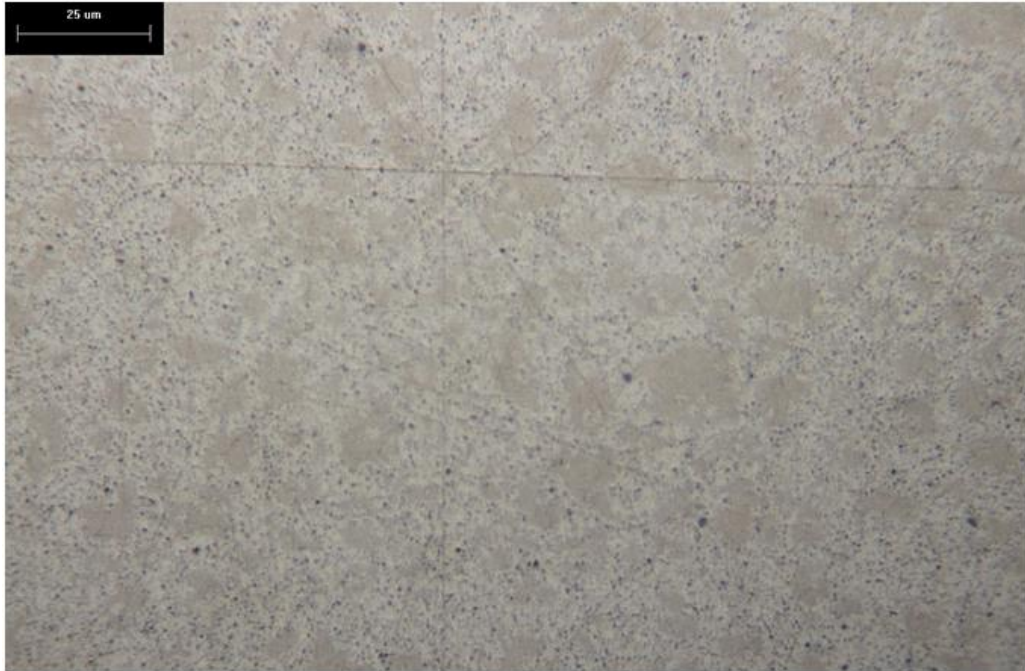
Figure 59. RERTR-8 Plate L1P020, mount 39W. Average fission density: 6.0 \times 10^{21} \text{ f/cm}^3 . Remaining grain structure can still be resolved optically.
