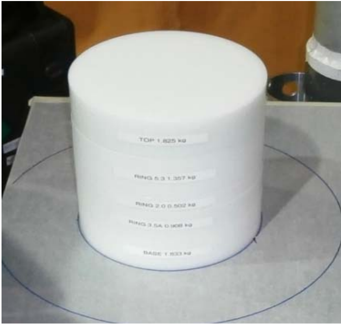
Fig. 3 Photographs of a configuration where two MARVEL core parts are separated by 2 cm of aluminum, and reflected with 5 cm of polyethylene. The upper image shows the HEU resting on one 5-cm thick disk of polyethylene, the lower photograph shows the assembly after the remaining polyethylene was placed around the HEU. The M value for this configuration was 6.04.
