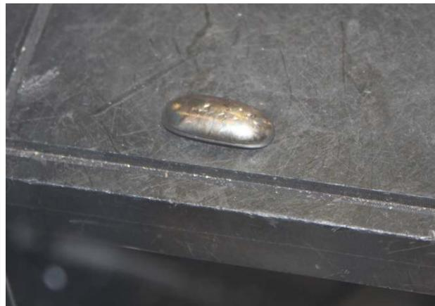
**Fig. 4.** Uranium Silicide Ingot after Arc Melting
