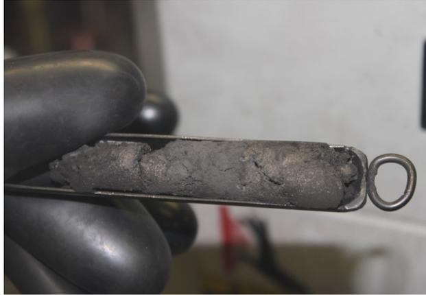
**Fig. 2.** Uranium from the Hydride/Dehydride Process
