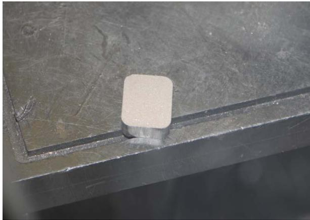
**Fig. 3.** Uranium and Silicon Compact before Arc Melting
