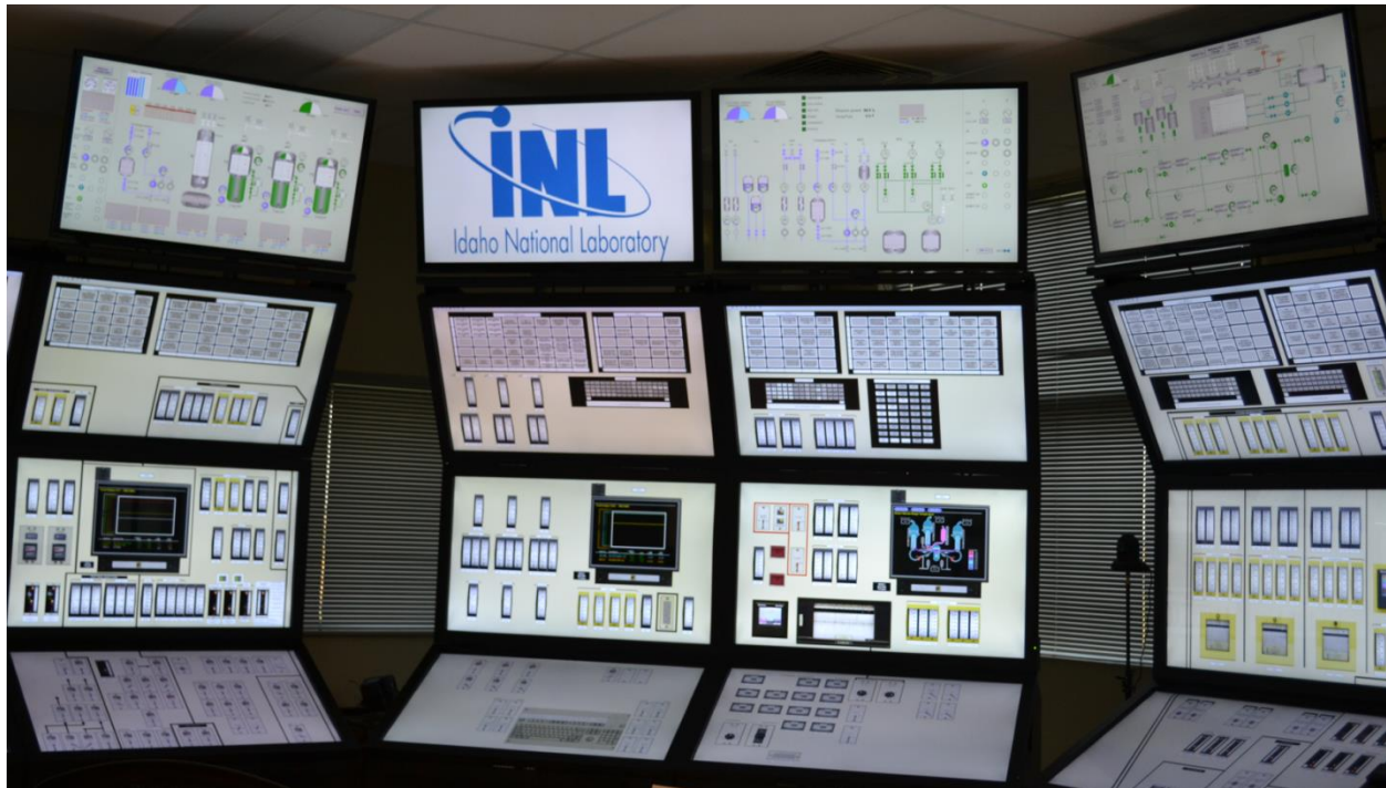
Figure 5. Layout of task-based overview displays in HSSL configuration.
