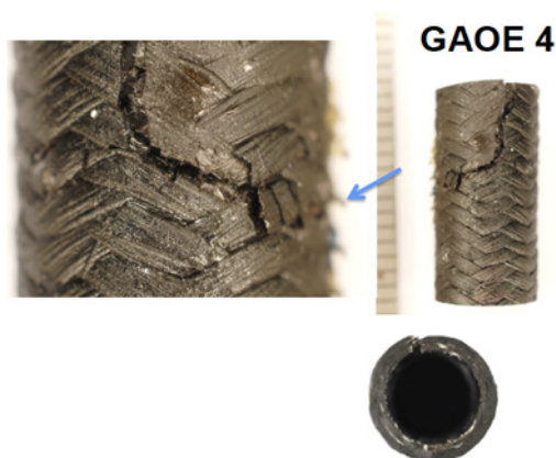
Figure 9. Oxidized burst testing of General Atomics Open Ended (GAOE) sample number 4.
