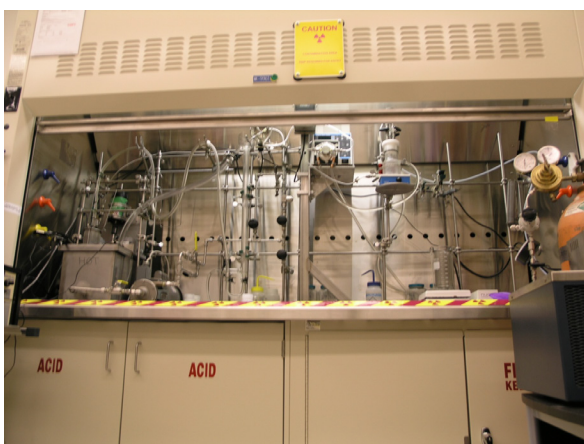
Figure 40. Internal gelation system used to make uranium gel spheres with carbon.
