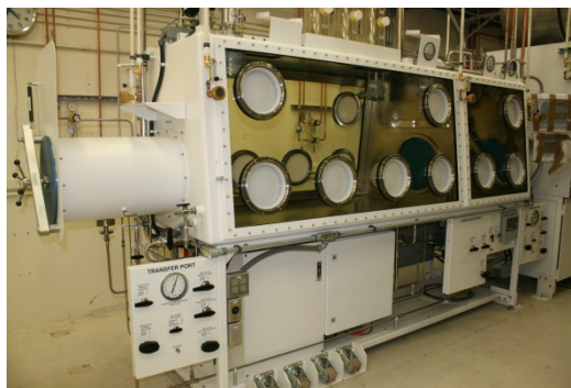
Figure 121. The TRU breakout glovebox was installed in Fuel Manufacturing Facility and factory acceptance testing was completed.
