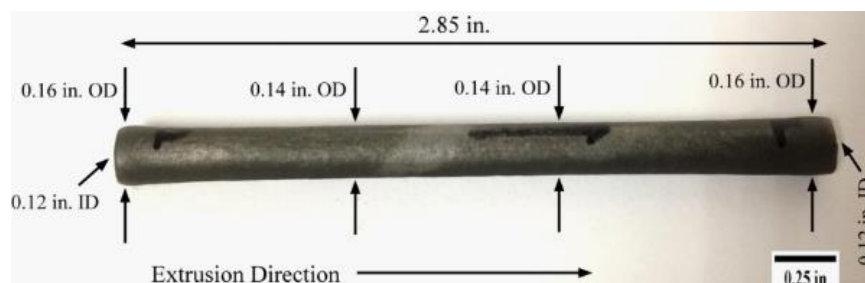
Figure 101. The FCRD-NFA1 tube was produced by hydrostatic extrusion at Case Western Reserve University.
