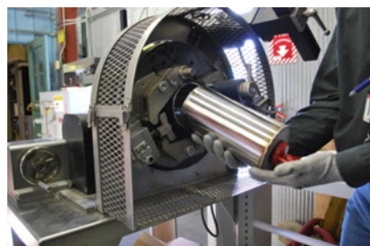
Figure 122. The 3013 can opener can be used to open the three nested cans in the 3013 storage container and will be placed in the TRU breakout glovebox.
