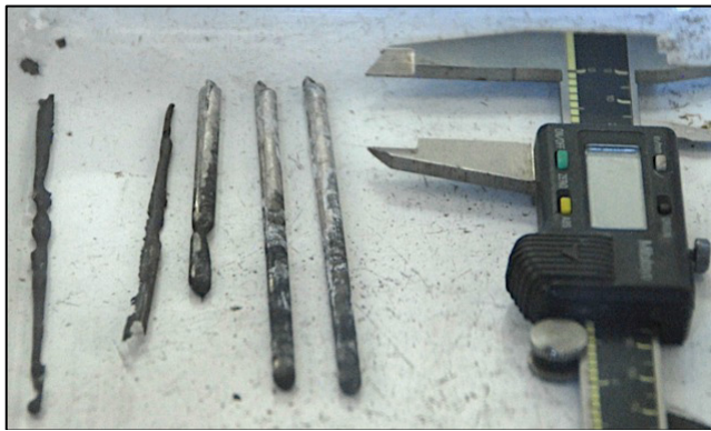
Fig. 2. U-TRU-Zr pins cast in the GACS (calipers set at 25.4 mm).
