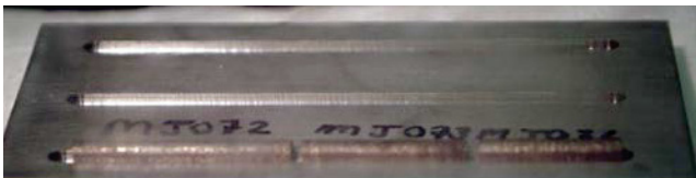
Fig. 2. Fuel column of the U-29Pu-4Am-2Np-30Zr composition prior to DOE-1 fuel pin loading.
