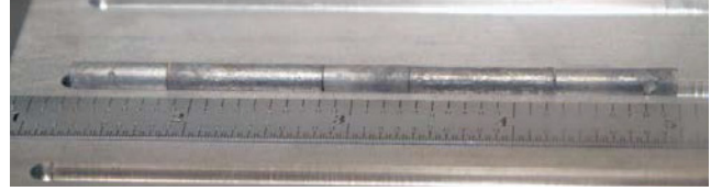
Fig. 3. Fuel column of the Pu-12Am-40Zr composition prior to DOE-2 fuel pin loading.
