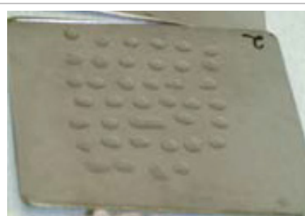
Figure 6. Stainless steel plate stippled with an ^{241}\text{Am} solution.
