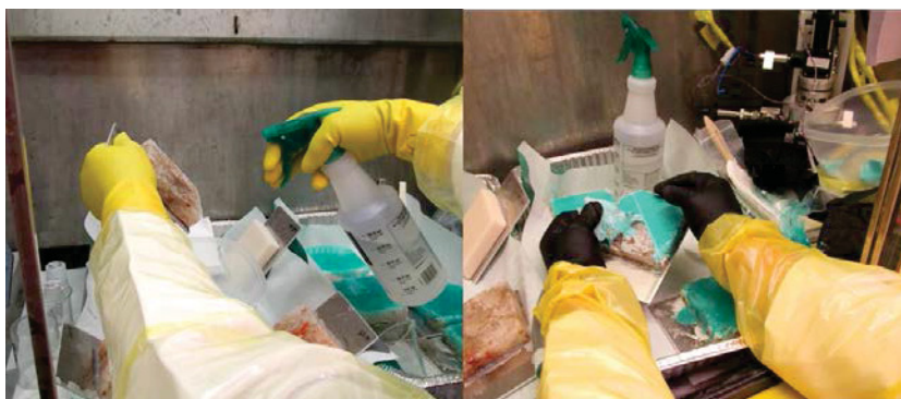
Figure 7. Left: Water washing americium from a salt coupon. Right: Removing DeconGel strippable coating from a salt coupon.
