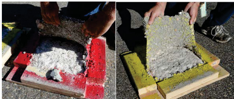
Figure 10. Rubble trays coated with Tekflex + PBS (left) and Tekflex + Stripcoat (right) after crush testing. The coating is manually peeled back to show that the integrity of the barrier was maintained under compression of the truck tire and under tension as the membrane is peeled away from the tray frame.
