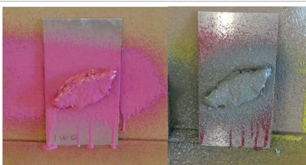
Figure 8. Application of PBS (left) and Tekflex (right) to a vertical surface. Note the propensity of the PBS coating to run during application.
