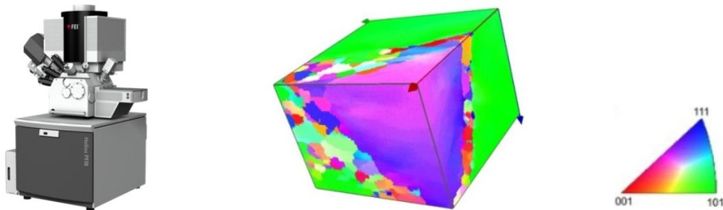
Figure 10. Left: a modern Helios PFIB microscope;<sup>4</sup> Right: 3D-representation of partial recrystallization in Al alloy.<sup>5</sup>
