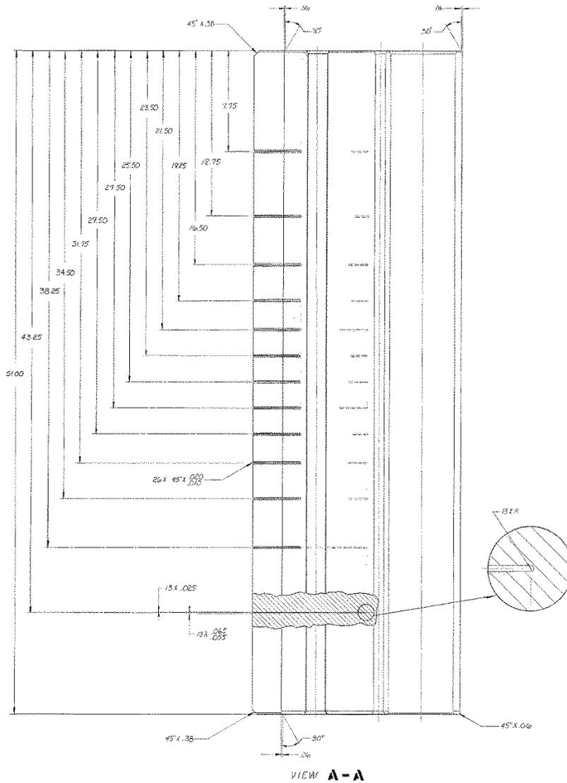
Figure 6. INL drawing DWG 419609 illustrating the geometry and arresting horizontal saw cuts of the beryllium reflector block(s) installed at ATR.
