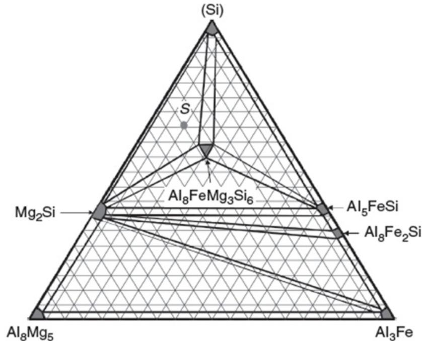
Figure 12. Isothermal cross-section in the  $\text{Al}_8\text{Mg}_5 - \text{Al}_3\text{Fe} - (\text{Si})$  pseudo-ternary phase diagram illustrating the character of phase equilibria in this complex system and phases that can potentially be present in AA6061.<sup>11</sup>
