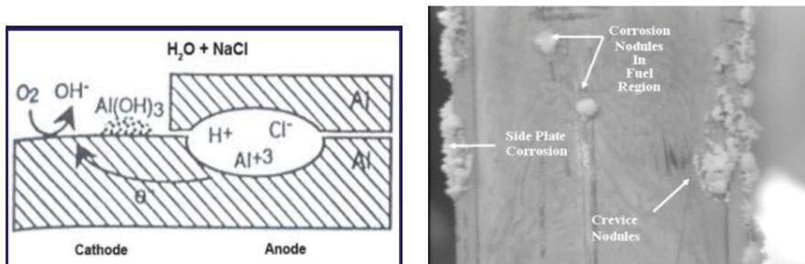
Figure 7. Schematic of crevice corrosion,<sup>1</sup> crevice corrosion at side plates in wet storage.<sup>2</sup>
