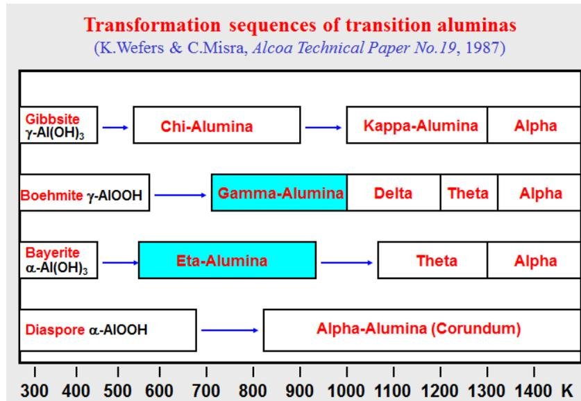
Figure 9. Crystallographic transformation sequences for different alumina polytypic structures.<sup>9</sup>
