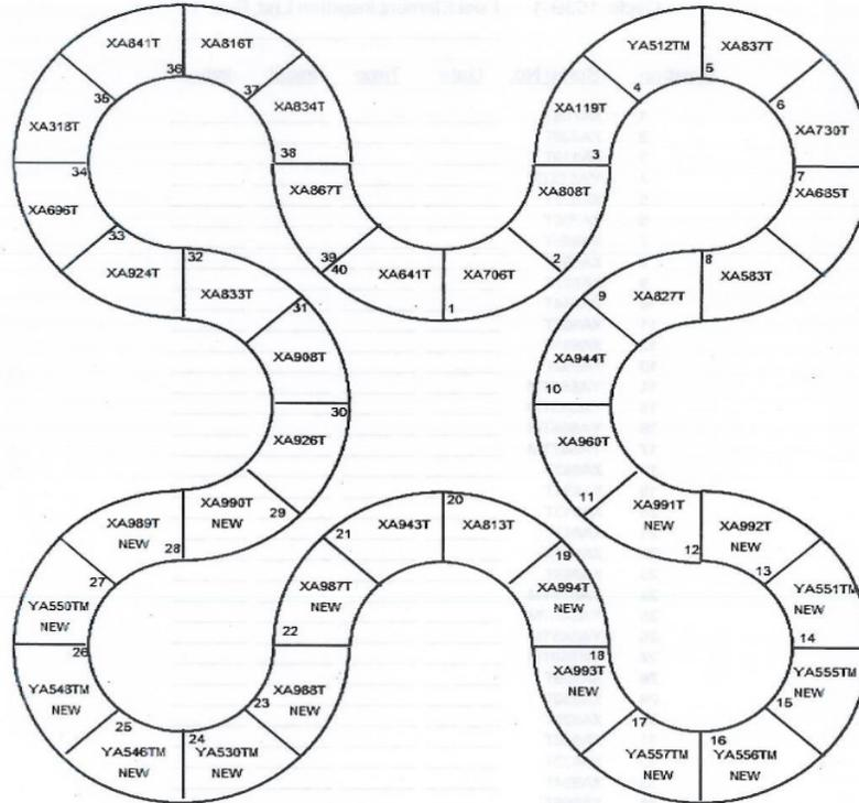
Figure 4. General configuration of the fuel elements in INL Advanced Test Reactor [9] (This core loading corresponds to fuel cycle 153B-1 studied in this report.)
