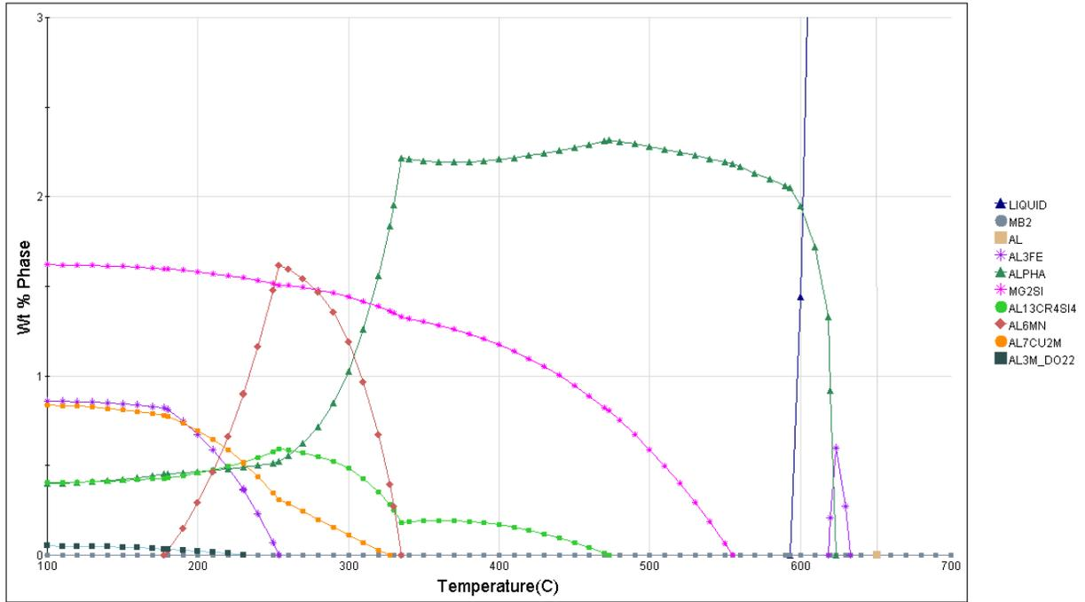
Figure 13. Temperature dependence for equilibrium alloy 6061 phase composition.
