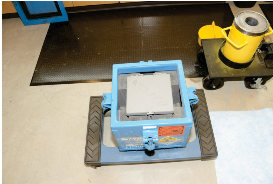
Figure 6. The shipping container (in blue) contains the specimens. Those specimens will be transferred to the yellow lead pig for storage and transport within the testing facility.
