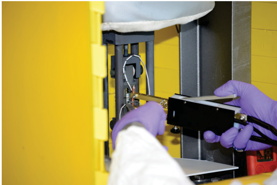
Figure 9. The direct current potential drop leads are being connected to the samples leads.
