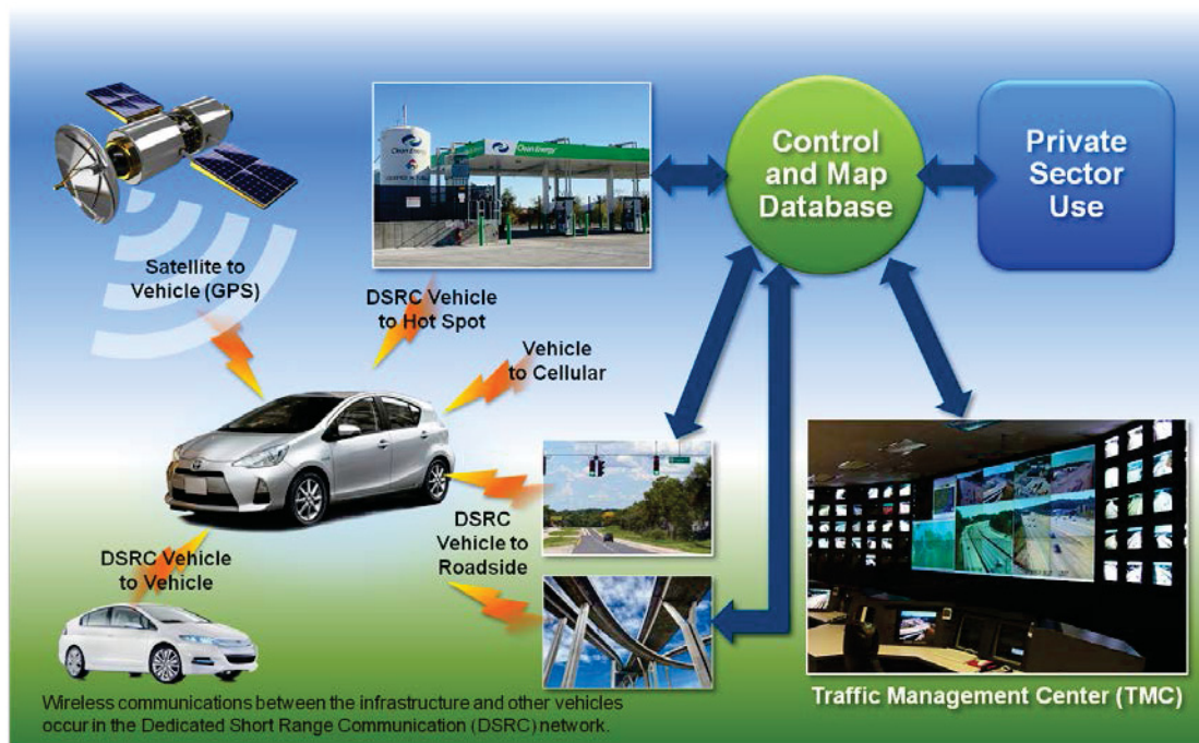
Figure 1. Overview of vehicle-to-vehicle and vehicle-to-infrastructure.
