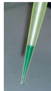
Figure 1. \text{UO}_2 dissolved in EMImFHF.
