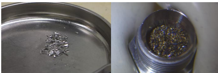
Figure 18. (a) Am metal just after distillation and (b) after storage in a Swagelok in the AFCI glovebox for approximately one month.
