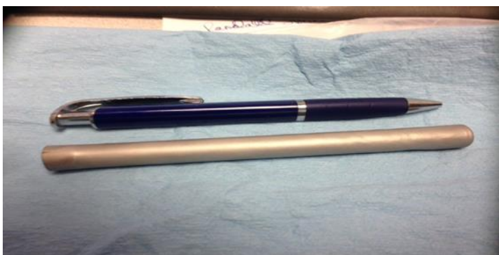
Figure 23. Thick-wall tube extrusion of 14YWT staged for pilgering.
