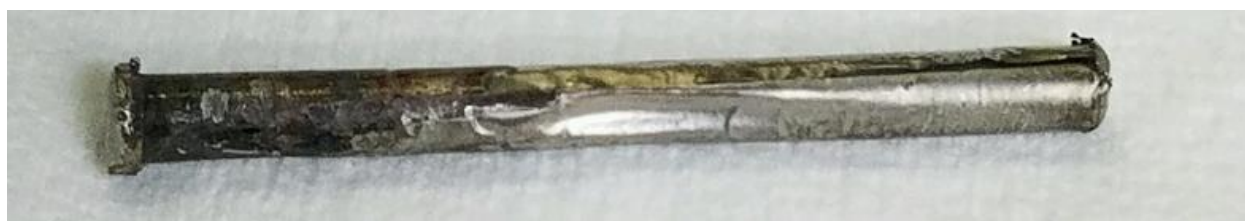
Figure 22. Degradation of the foil throughout the length of the pin.
