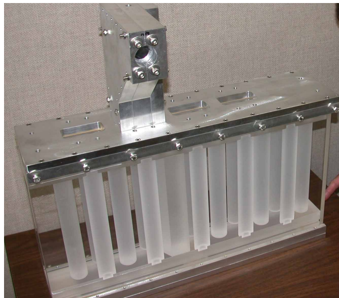
Figure 4. Photograph of the scaled model used in the INL MIR facility to obtain flow data. Inlet flow must negotiate a 90° -bend just prior to entering the flow section.
