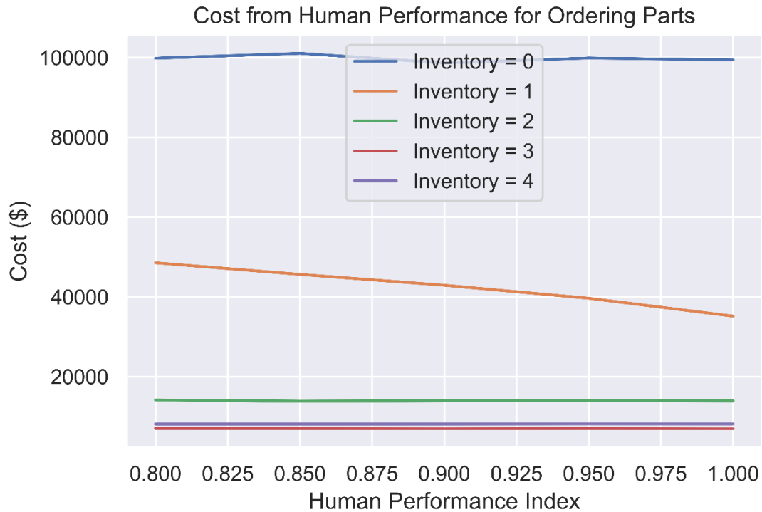
Figure 74. Costs for ordering parts as a function of human performance rate and available inventory.
