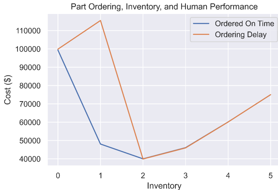
Figure 76. Cost for ordering parts as a function of mistiming ordering and available inventory.
