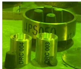
Low dose rate, small size HALEU metal regulus
