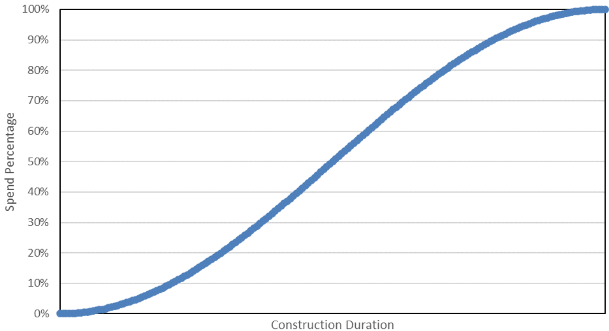
Figure 20. Example construction spend curve.
