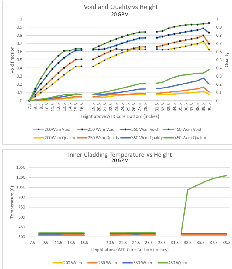
Figure 15. Void fraction, quality values, and inner cladding temperatures over the length of the three fueled test train tiers (20 gpm).
