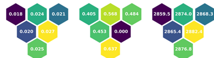
Figure 25. Mass flow rates (left) in kg/s, orifice diameter in cm (center), and max fuel temperature in K (right).
