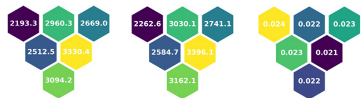
Figure 23. Propellant exit (left) and max fuel (center) temperatures in K, and mass flow rates in kg/s (right) with no orifices.
