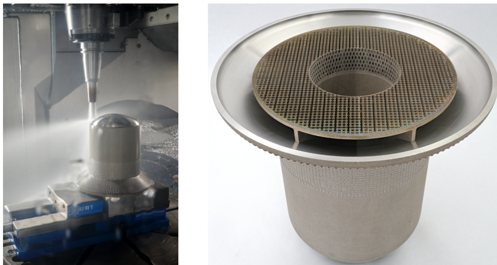
Figure 7. Ongoing effort by the AMMT program to 3D-print a liner for MARVEL. At left, final machining of the additively manufactured component, and at right, a finished reduced-scale piece. Credit: ORNL.
