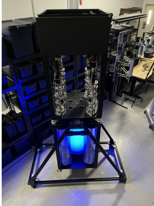
Figure 8. MACS, used as a non-nuclear replica of MARVEL for controls testing [Farber 2023].
