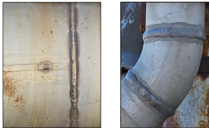
Figure 1. Examples of sensitization occurring in the heat affected zone in stainless steel components. Dark regions adjacent to the welds are areas of accelerated corrosion due to carbide precipitation during welding.
