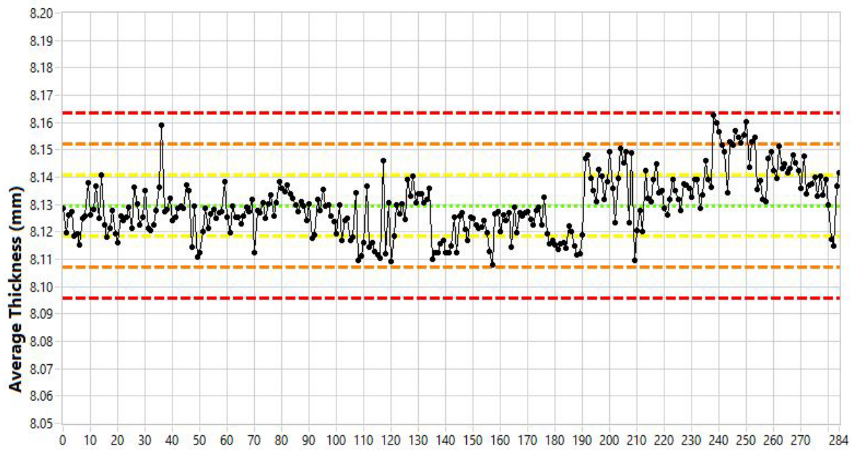
Figure 15. Average thickness (mm), mean = 8.1296, standard deviation = 0.0113, COV = 0.14%.
