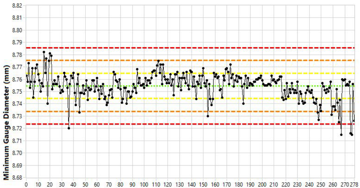
Figure 23. Minimum gauge diameter (mm), mean = 8.753, standard deviation = 0.01, COV = 0.11%.
