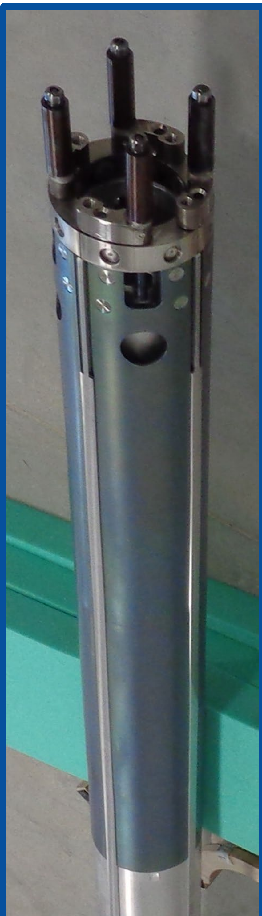
Figure 2: Picture from the recent CIC showing a fully assembled safety rod.
