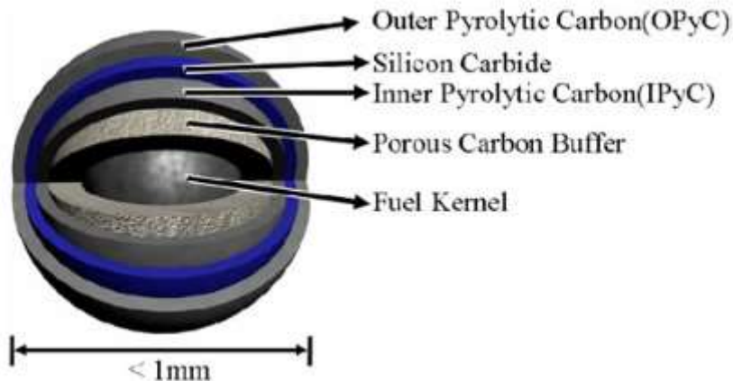
Figure 2. Schematic of a TRISO fuel particle [4].
