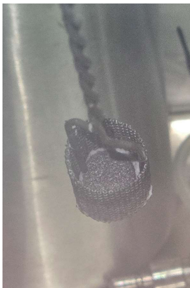
Figure 8. SiC sample A after removal from the furnace.
