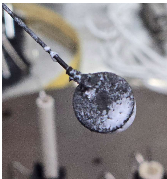
Figure 10. SiC sample B with stainless-steel wire lead.
