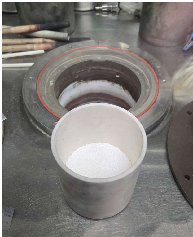
Figure 4. Alumina crucible containing LiCl-KCl- \text{MgCl}_2 salt in front of the furnace used for testing of the EMS-CC process.
