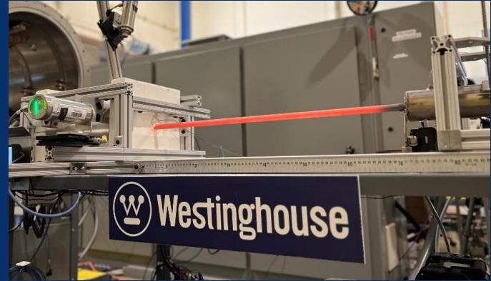
Top: Full-Size Graphite Core Block Bottom: 4 ft Heat Pipe Testing
