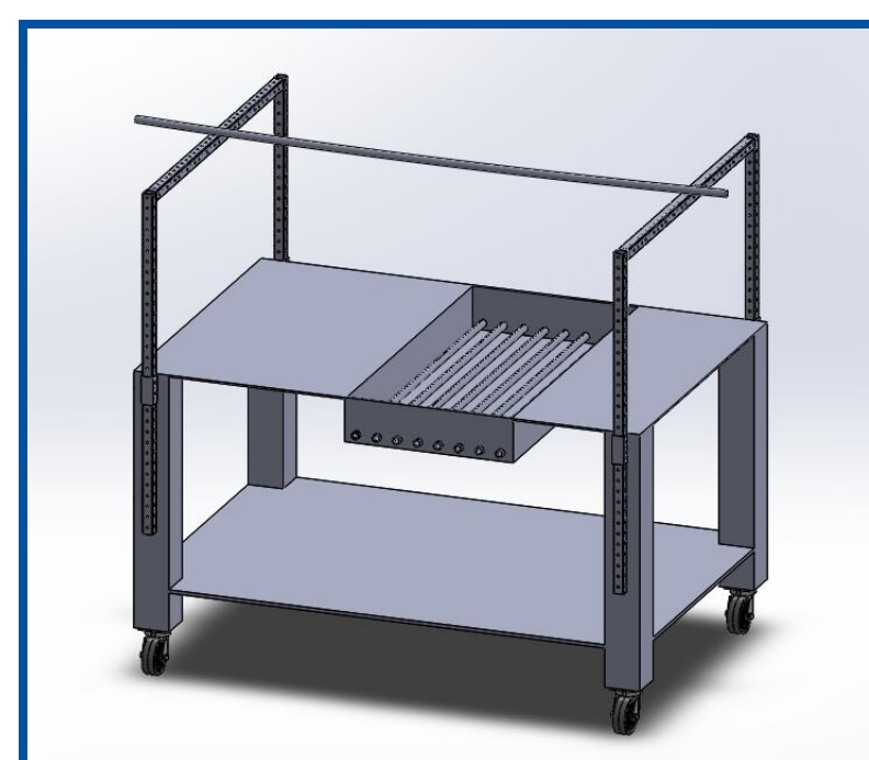
Figure 3: Preliminary fire test table design as created in SolidWorks (computer aided design) software 3
