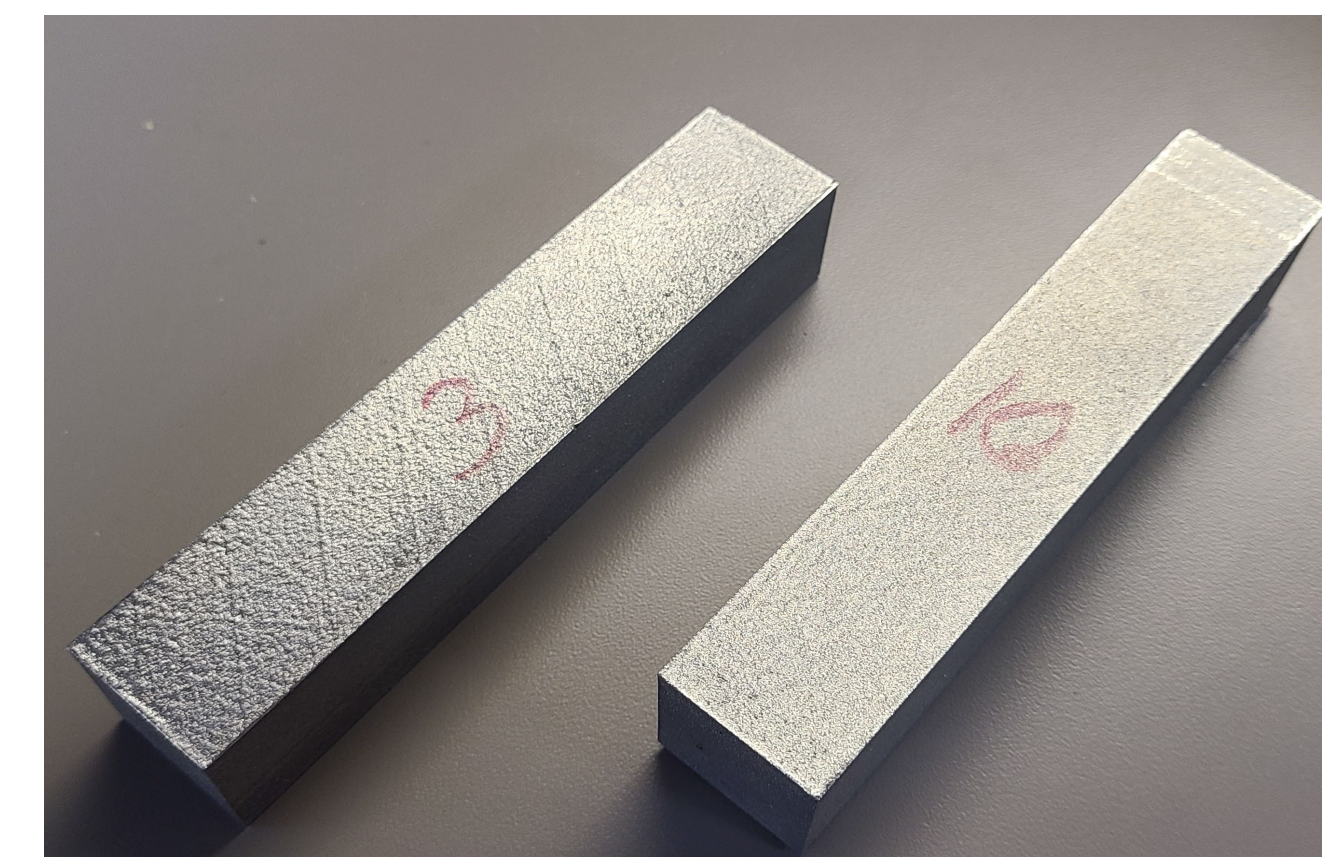
Figure 2. LANL LPBF 316H SS square bars (i.e. "loaves"), featuring loaves #3 and #10
