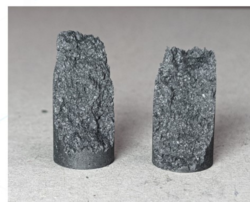
Figure 1: Fractured PCEA-grade graphite specimen after SHPB test.
