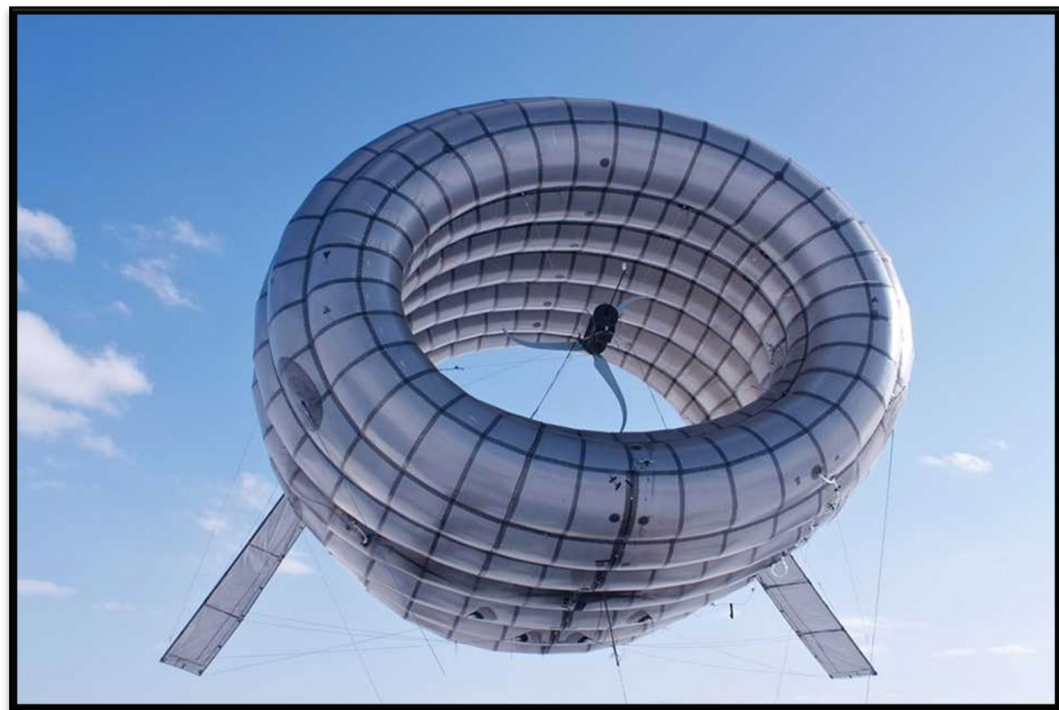
Altaeros Energies' BAT floats 1,000 to 2,000 feet high to harness stronger winds (MIT News)
