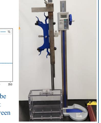
As shown above, the pressure readings from dip-tube one and dip-tube two are similar. This is to be expected as both dip-tubes are placed at nearly the same height in the fluid. The differences in pressures between these two tubes is a result of the differences in tube inside radii
