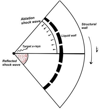
Schematics of the gas dynamics within the chamber
