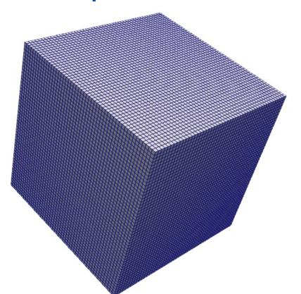
A finer mesh leads to a better match between the simulation prediction and the analytical solution
