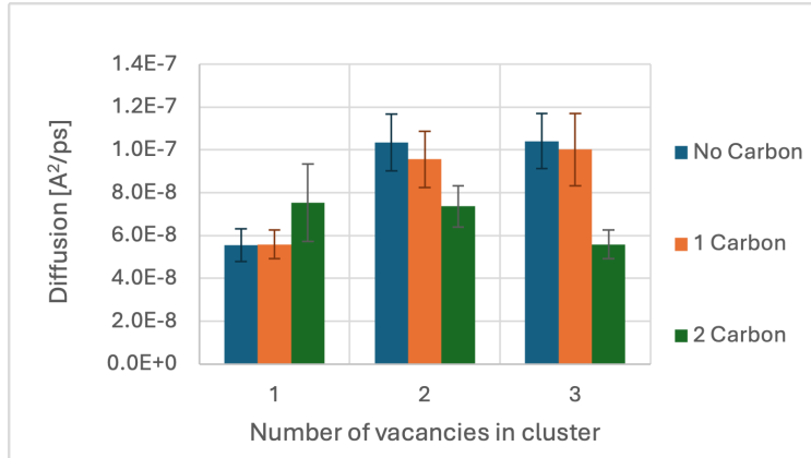
Figure 15. Measurement of the total diffusion induced in a model Fe-Cr-C system due to the placement of a small vacancy cluster, with up to two carbon atoms added in close proximity.
