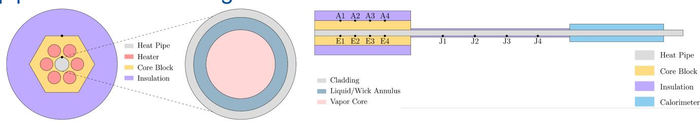
The temperature distribution was obtained by thermocouples located in the core block, evaporator, and adiabatic section.
