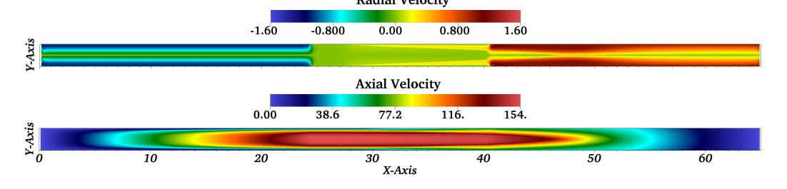
An annular-wick heat pipe was used as a code **VALIDATION**Experiments conducted at the SPHERE facility at INL [1] validated the heat pipe temperature distribution. The setup consists of a 7-hole hexagonal core block with a central heat pipe and 6 surrounding heaters.
