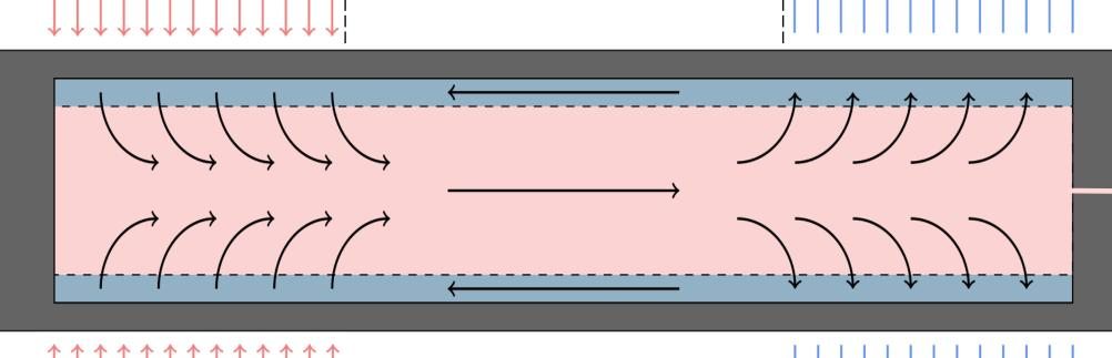
A cross-section of the vapor core of a heat pipe, using LES in Nek5000, shows the transition to turbulent flow between the end of the adiabatic section and the beginning of the condenser section as the vapor condenses.
