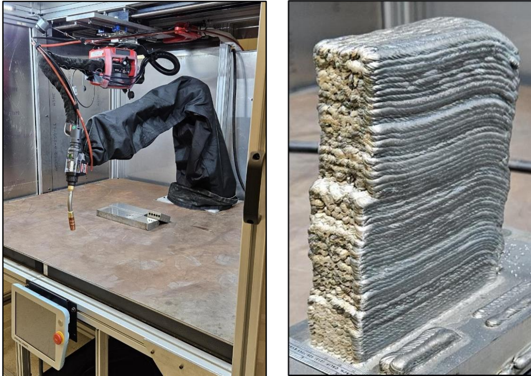
Figure 3. Photo of the robotic welding setup for wire arc additive (left) and the completed GMA-DED block (right).
