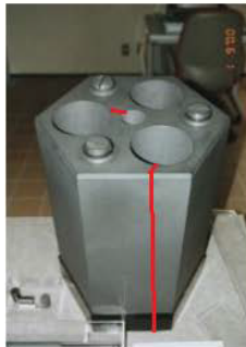
Figure 2: Illustrative example of cracking in a prismatic HTGR block
