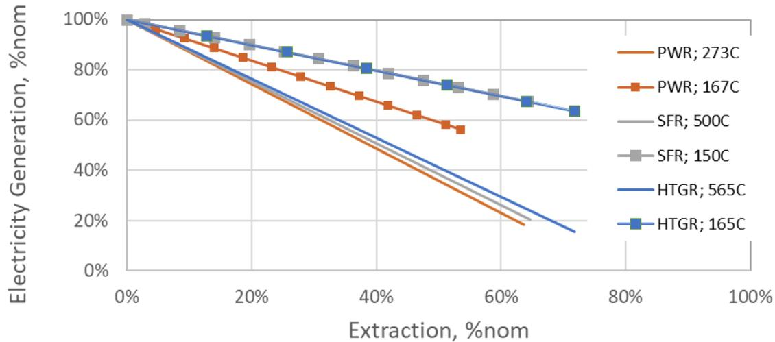
Figure 14. Relationship between steam extraction for non-grid applications and the resulting decrease in electricity generation [33].
