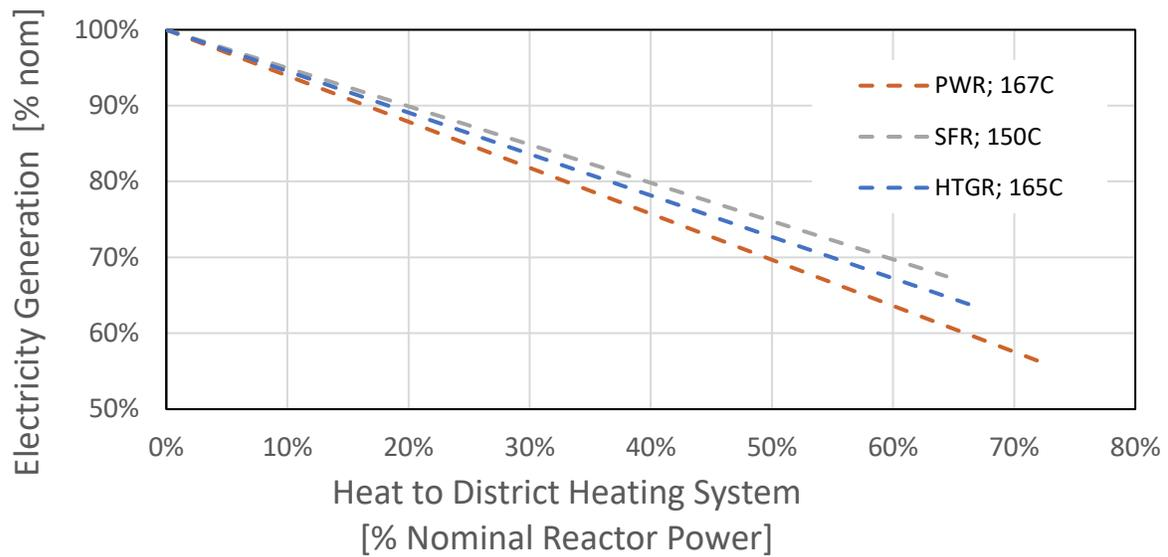
Figure 15. Heat extraction for district heating.
