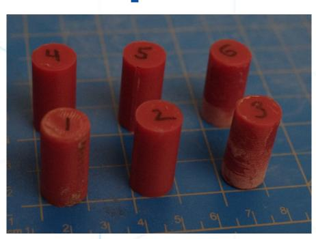
Figure 6: Irradiated compression samples
