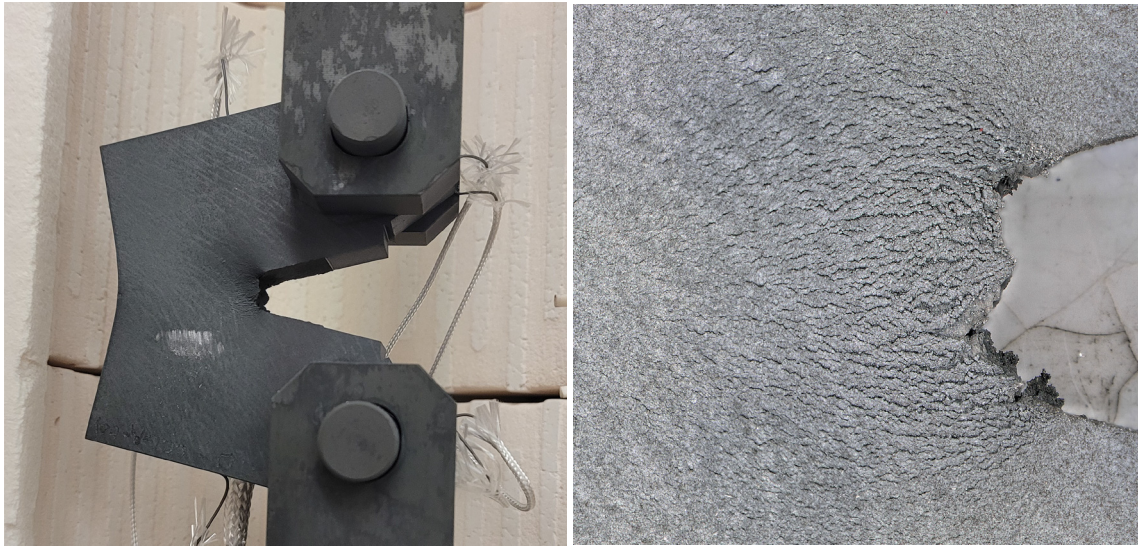
Figure 6. Alloy 709 CCGR, Test 1, CT specimen after termination of the test. Higher-magnification image of the notch tip is shown on the right.
