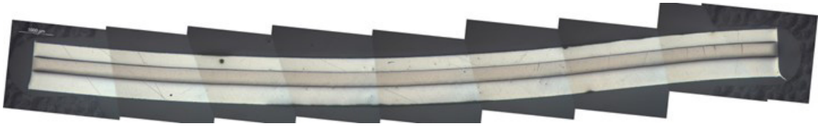
Figure 26. Metallography image from top edge of fuel zone. Fission density \sim 1.5\text{E}+21 fissions/cm 3 .
