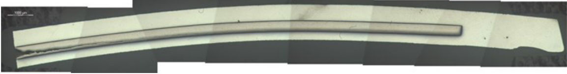
Figure 45. Metallography image 7 cm from bottom of fuel zone. Fission density \sim 2.0\text{E}+21 fissions/cm 3 .
