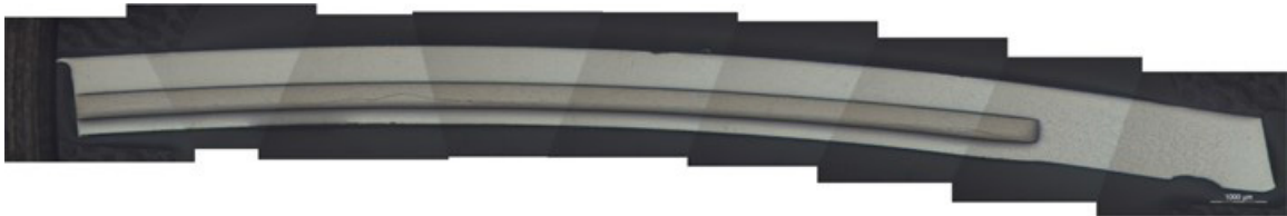
Figure 28. Metallography image from fuel centerline. Fission density \sim 2.7\text{E}+21 fissions/cm 3 .
