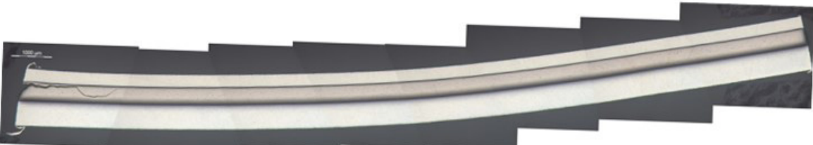
Figure 42. Metallography image from plate mid line. Fission density \sim 2.8\text{E}+21 .
