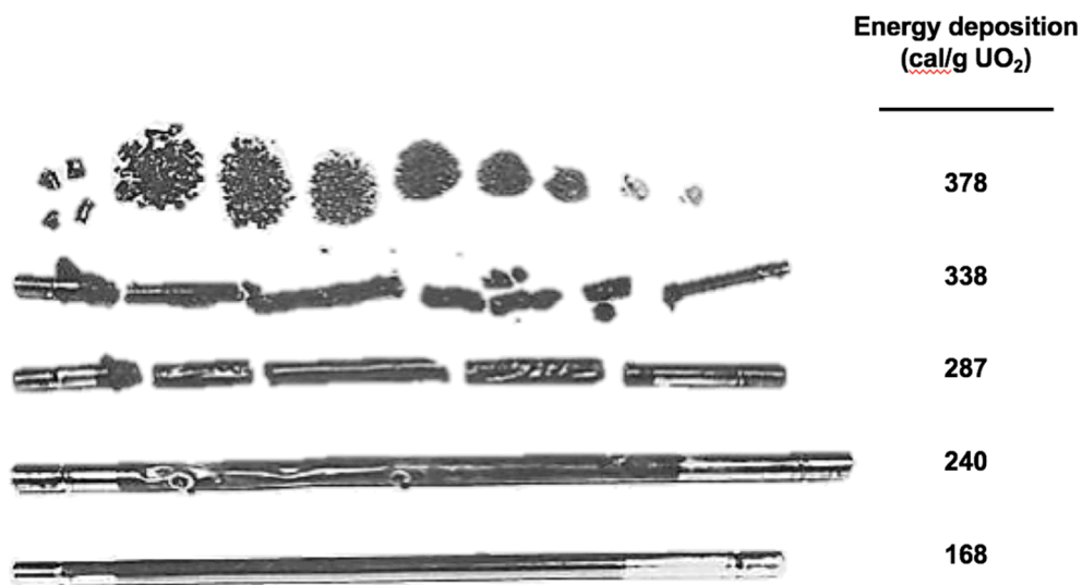
Figure 6. Pictures of failed fuel following RIA testing in SPERT.
